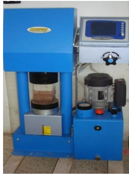
Fig.A-3. Compressive strength test of the units
