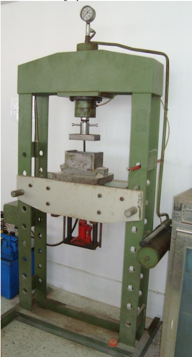
Fig.A-2. Bench model, semiautomatic press machine
