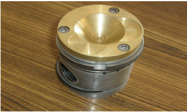
Fig 1: Aluminum crown with an air-gap insulated piston with brass insert
