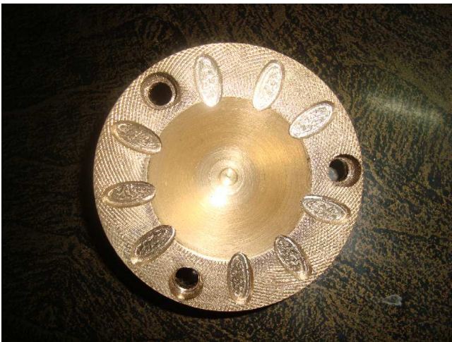
Fig: 6 Photo Graphic View of Brass Crown Piston with 9 Grooves
