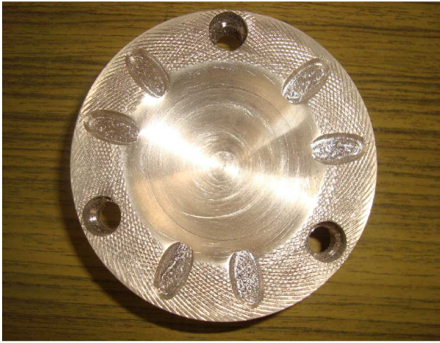
Fig: 5 Photo Graphic View of Brass Crown Piston with 6 Grooves
