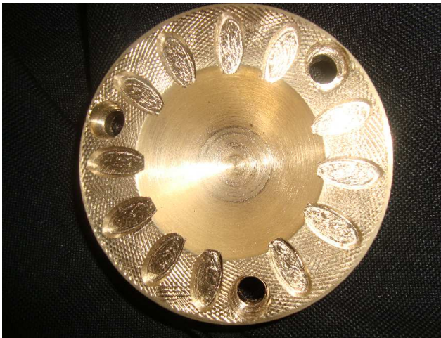
Fig: 7 Photo Graphic View of Brass Crown Piston with 12 Grooves
