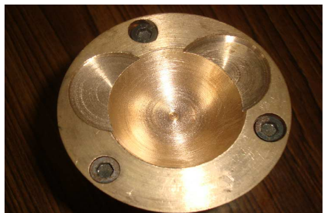
Fig 4 Photo Graphic View of Plain Brass Crown piston
