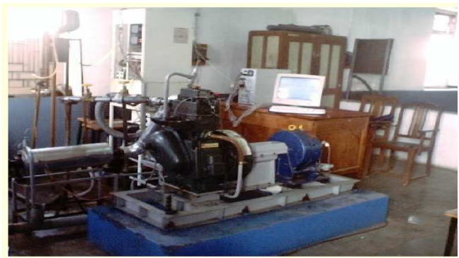
Fig. 3. Experimental set up of Insulated Engine Test Rig
