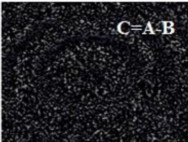
Fig.6 Speckles (Before & after) with Subtracted fringe Pattern
