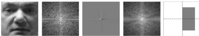
Figure 3.2 Two-Dimensional Discrete Fourier Transform of a Face Image :The Real part(log plot),the Imaginary part, and the Magnitude in Fourier domain
