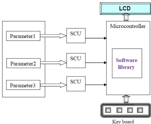
Figure 1. Block diagram of microcontroller interfacing system
