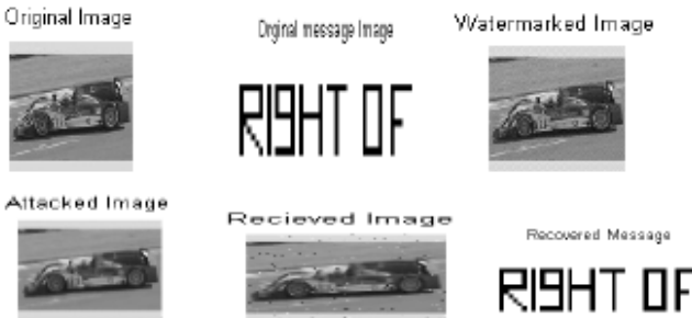
Figure 8(c) Watermarked Image with median attack with PSNR = 21.3140 dB and Compression Ratio = 66.6176
