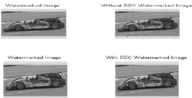
Figure 8(l) Watermarked image with Error Correcting code (Cyclic Code) with PSNR = 62.2016 dB and Compression Ratio = 66.61
