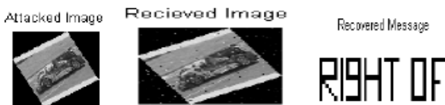
Figure 8(h) Watermark image without Error Correcting code with PSNR = 37.8631 dB and Compression Ratio = 66.6176
