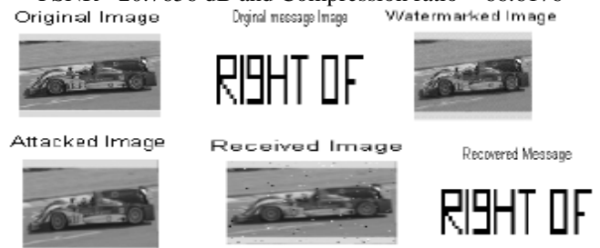
Figure 8(c) Watermarked Image with blurring attack with PSNR = 20.7656 dB and Compression Ratio = 66.6176
