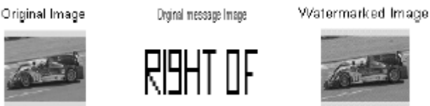
Figure 8(c) Watermarked Image with rotation attack with PSNR = 11.4951 dB and Compression Ratio = 66.6176
