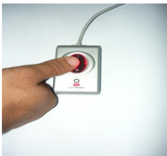
Fig 5: The incorrect method to place a finger on the device [5]
