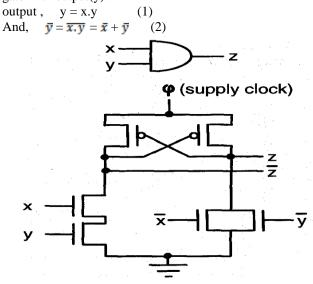
Figure 4. ECRL and gate circuit
