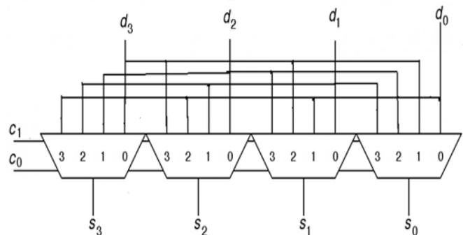
Figure 8. 4-bit barrel shifter circuit
