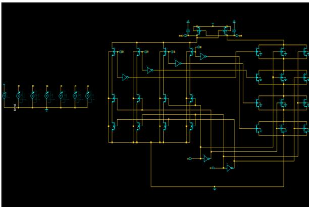
Figure 11. 4 input multiplexer schematic
