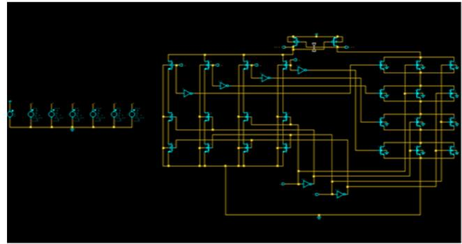
Figure 6. Implementation Schematic 4.1 multiplexer using ECRL technology
