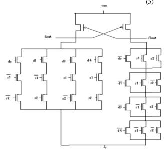
Figure 5. ECRL multiplexer circuit
