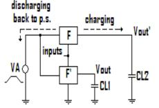
Figure 2 Charging and Discharging in Adiabatic system Figure 2 shows the Charging and Discharging in Adiabatic System. In figure F functional block use PMOS transistor and FBar use NMOS transistor. Ease of Use
