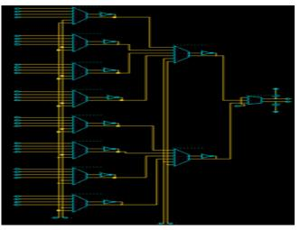
Figure13. 32 input multiplexer Schematic
