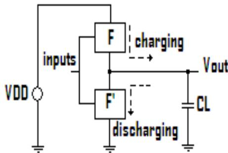
Figure 1 Charging and Discharging in CMOS System
