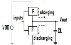
Figure 1 Charging and Discharging in CMOS System
