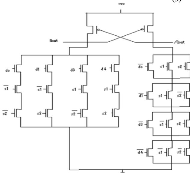
Figure5. ECRL multiplexer circuit
