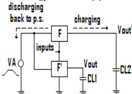
Figure 2 Charging and Discharging in Adiabatic system
