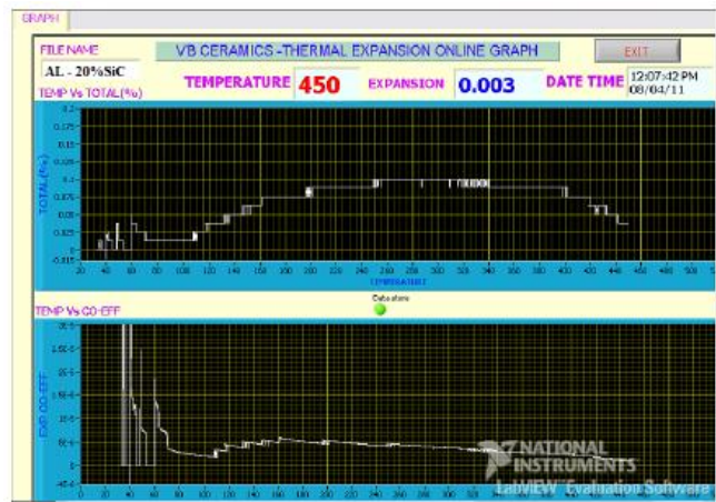
Figure 16. Co-efficient of Thermal Expansion for Al – 20%SiC
