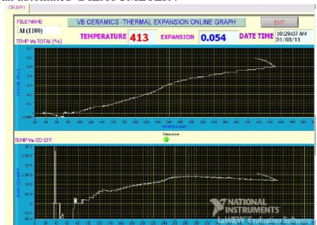
Figure 12 Co-efficient of Thermal Expansion for Pure Al
