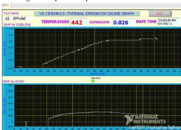
Figure. 15 Co-efficient of Thermal Expansion for Al – 15%SiC
