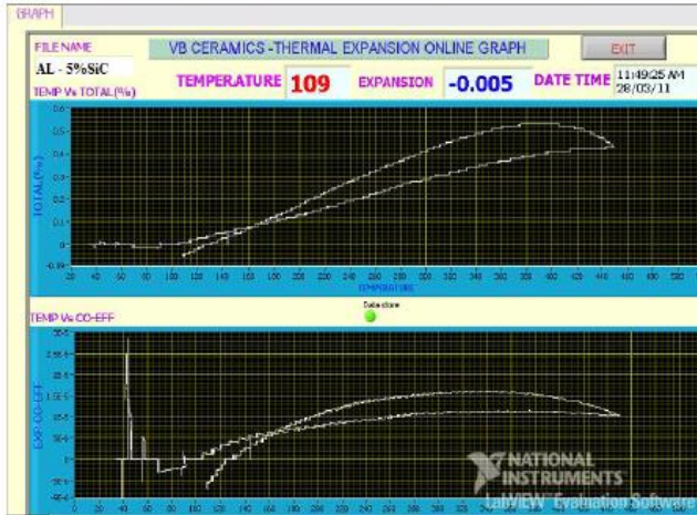
Figure 13 Co-efficient of Thermal Expansion for Al – 5%SiC From the Fig.13, the total percentage of thermal expansion gradually increases up to 0.043 \mu\text{m}/\text{m}\cdot^\circ\text{C} for 5% SiC by increasing the temperature up to 450 ^\circ\text{C} .
