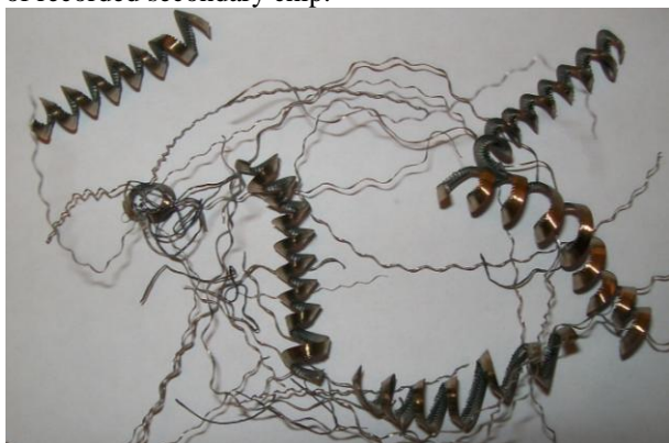
Fig. 14 View of the recorded primary and secondary chip
