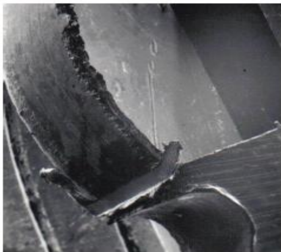
Fig. 12. View of the process of chip creation from the tool side
