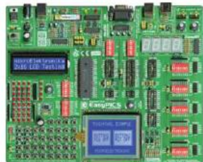
Fig (8) EASYPIC5 microcontroller development Board
