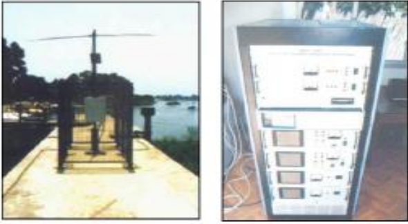
Fig (2) Meteor- Burst Sub And Base Station
