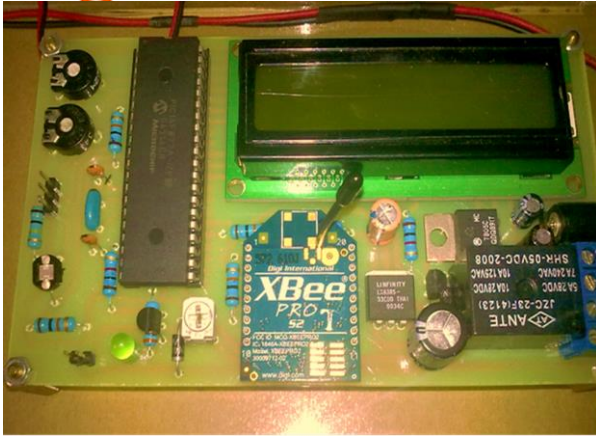
Figure 3: ZigBee based wireless local station
