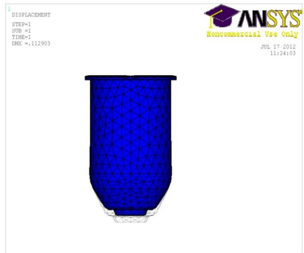
Fig 10: Deformation in the filter bowl 0.1123 mm
