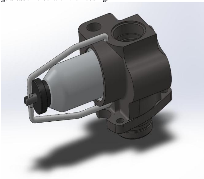
Fig 3: Assembly drawing of feed pump
