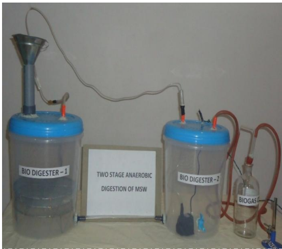
Photograph -2 Working setup of two stage anaerobic digestion system
