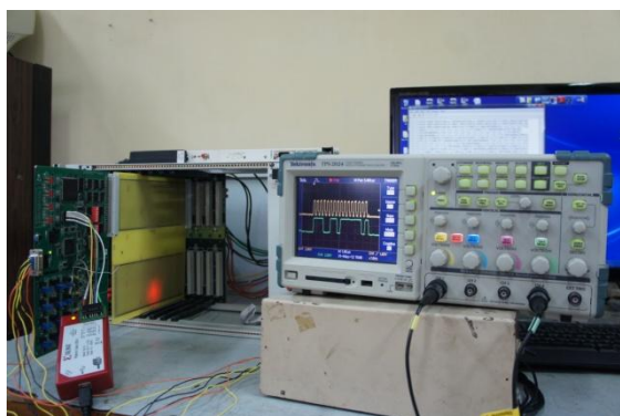
Figure 10 : ADC Card Attached in VME Crate
