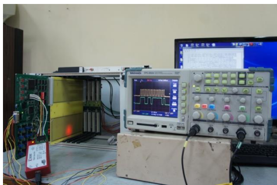
Figure 10 : ADC Card Attached in VME Crate
