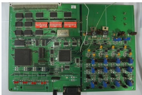
Figure 9 : Four Channel ADC Card
