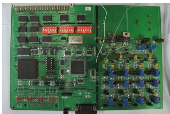
Figure 9 : Four Channel ADC Card
