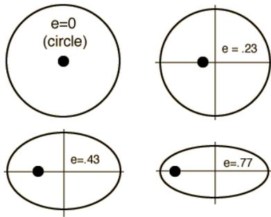
Figure 2: elliptical paths with varying eccentricities
