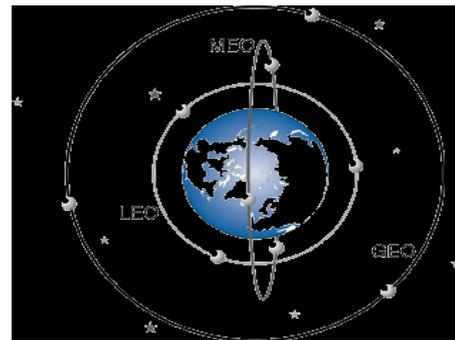
Figure 1 : This explains about the altitudes of GEO , MEO , LEO
