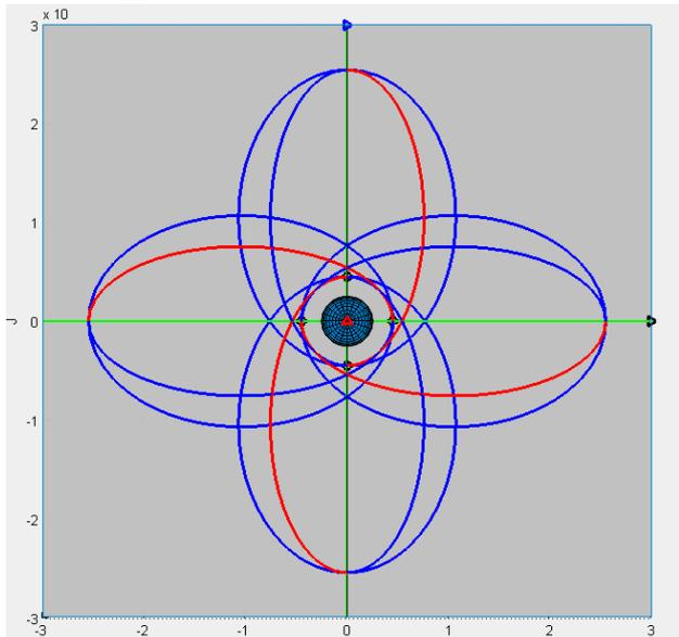
Figure-15: view all the orbits in the four quarters of the planet , which includes GEO , MEO . each quarter part of the planet has 3 orbits ( one GEO + two MEO )
