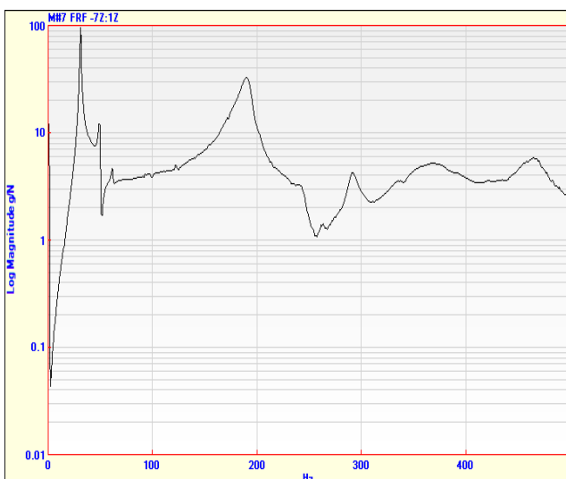
Fig – 3 Kevlar- cantilever condition
