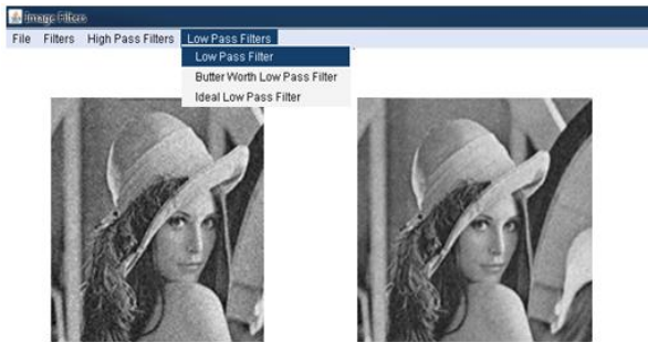
Figure 1: Illustrating the low pass filter removing the noise from the foreground
