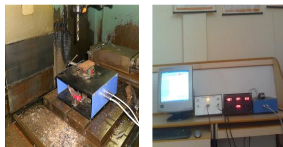
Photo 1- Experimental Setup for Mechanical Load
