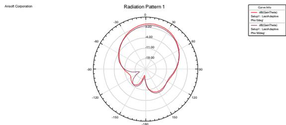
**Fig12: Radiation pattern of Gain in Theta direction.**
