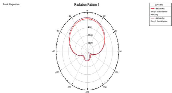
**Fig13: Radiation pattern of Gain in Phi direction.**
