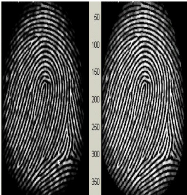
Fig. 4.2.2(b) Histogram Enhancement. Original Image (Left). Enhanced image (Right)
