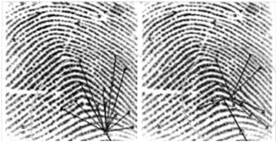
Fig. 2(a) Size of a bounding circle is large if the reference point is near boundary (b) Size of the bounding circle decreases when a "centralized" reference point is used.
