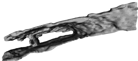
Figure 5. SR4000 data visualization using a ray-carving technique (Gold Reef City Mine)
