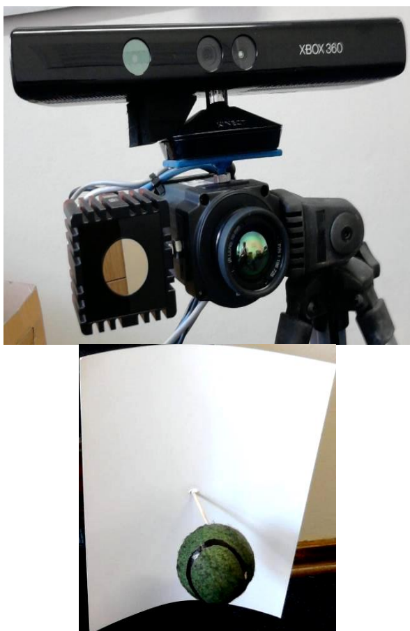
Figure 7: Multi-sensor setup with SR4000 TOF camera, FLIR A300 IR camera and XBOX Kinect rigidly mounted on a tripod (left), and tennis ball calibration object (right)
