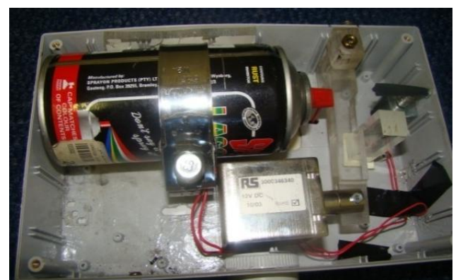
Figure 7: Prototype WSA head – wall exciter (solenoid); spray nozzle extender; enclosure; ESD; mechanical lever; solenoid for the spray mechanism.
