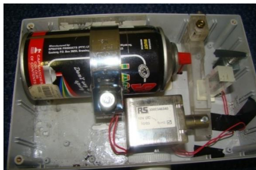
Figure 7: Prototype WSA head – wall exciter (solenoid); spray nozzle extender; enclosure; ESD; mechanical lever; solenoid for the spray mechanism.
