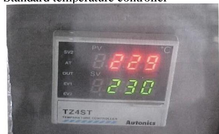
Fig 6.3 Existing system for Temperature Control
