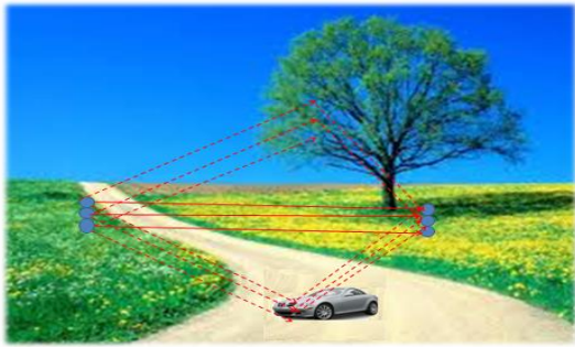
Fig 2. In MIMO Each Virtual multipath route is treated as a separate channel
