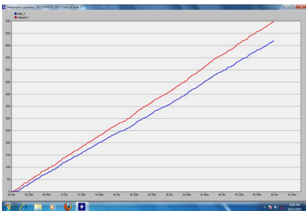
Fig 2: shows the Number of request Arrived (red) in network and numbers of file delivered (blue) to nodes when ultra peer formation enabled.
