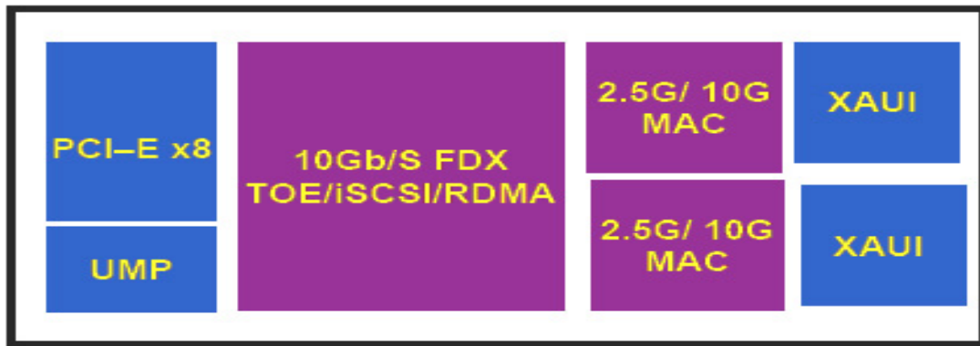
Fig. 1. Block diagram of the Broadcom 57710 controller 2
