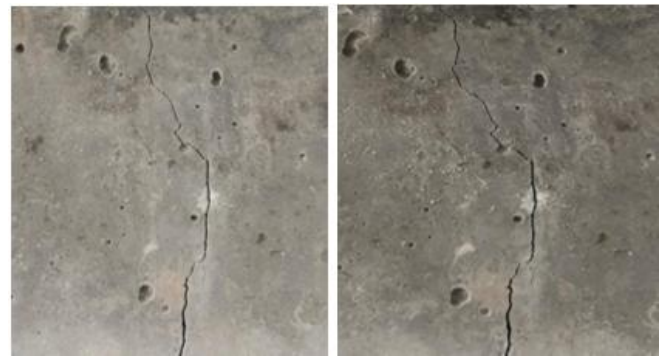
[Fig.5: Cracks on Ordinary Concrete Before and After 35 Days]
