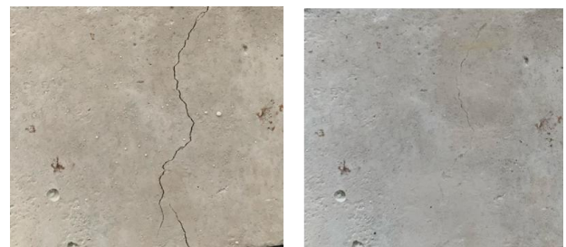
[Fig.6: Cracks on Concrete Made with Silica Fume Before and After 37 Days]
