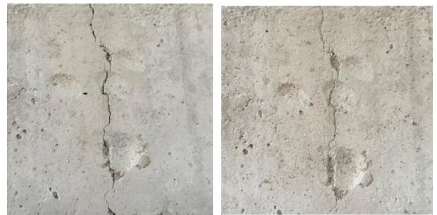
[Fig.7: Cracks on Concrete Made with Silica Fume, Along with Sap Before and After 21 days]
