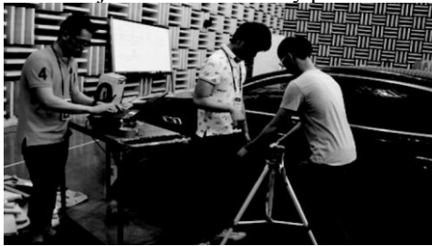
Fig. 10. Noise Recording in Anechoic Chamber [6]
