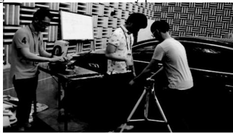
Fig. 10. Noise Recording in Anechoic Chamber [6]
