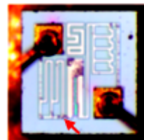
Figure-10: Discontinuity of thin film track of resistor R9
