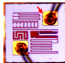
Figure-12: Discontinuity of thin film track of resistor R15
