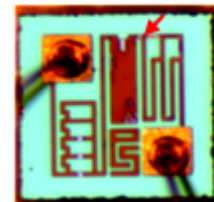
Figure-11: Discontinuity of thin film track of resistor R12
