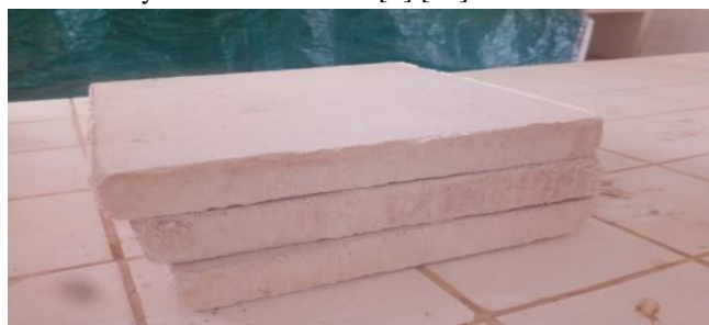
Fig. 7. Picture of samples of diatomite bricks
