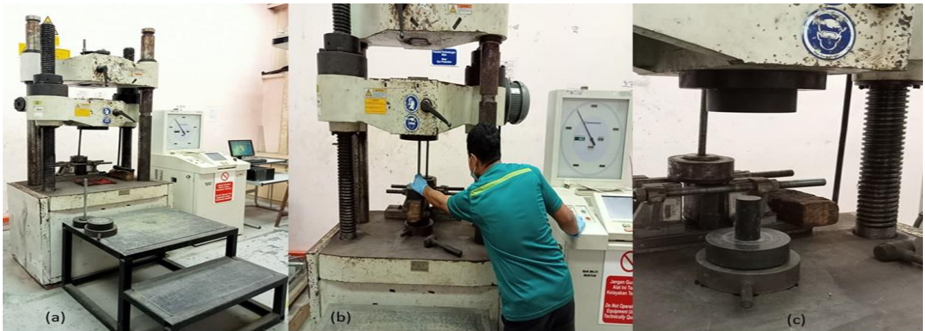
Fig. 2. Compression test set up. (a) Overview of testing machine. (b) Preparing the top and bottom compression plates. (c) Placement of test sample on testing machine.
