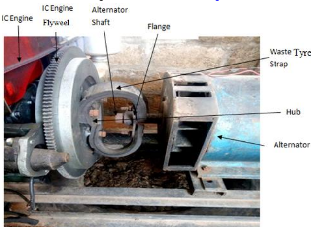
Fig. 2 Waste tyre coupling system test arrangement
