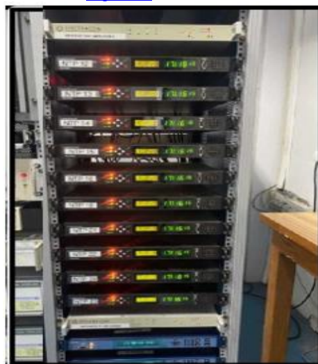
Fig 4: Figure represents the stack of NTP servers providing NTP services at NPLI. These servers provide the time over internet using NTP
