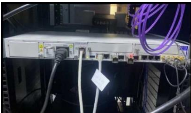
Fig 10: Stratum 1 NTP server at Hyderabad site
