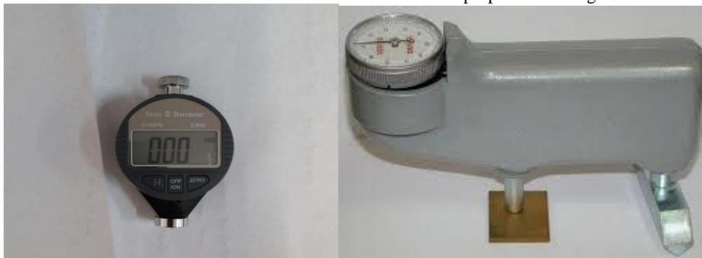
Fig. 10 Shore-D & Barcol Hardness Testers
