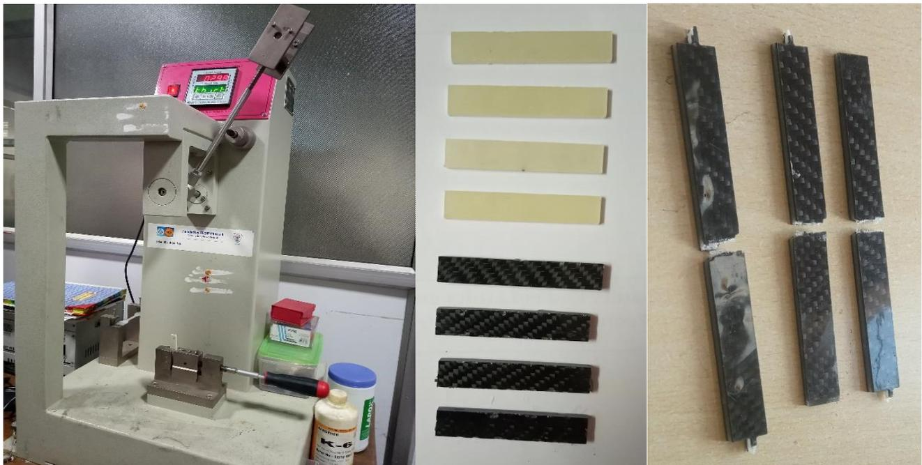
Fig. 9. Specimen under Impact Test & Failed Specimens
