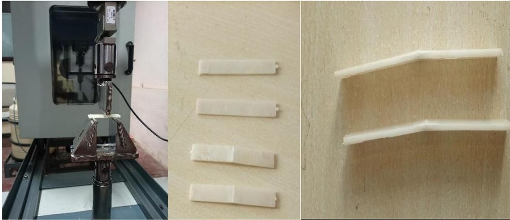
Fig. 8. Specimen under Flexural Test & Failed Specimens
