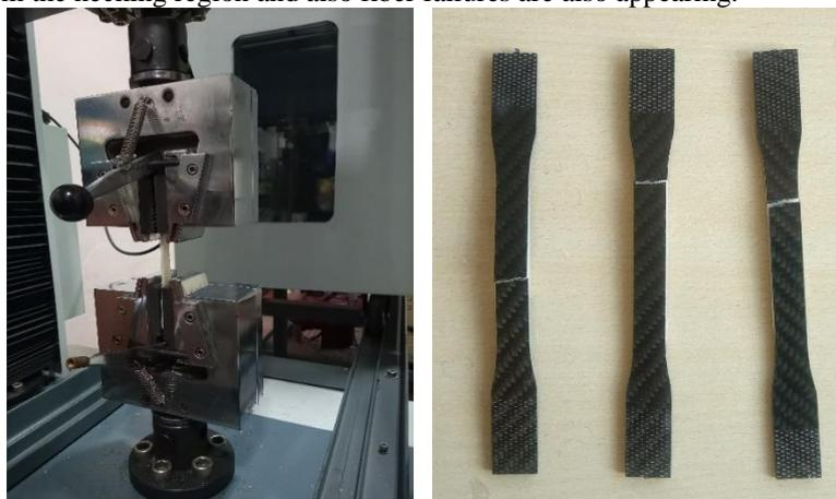
Fig. 7. Specimen under Tensile Test & Failed Specimens
