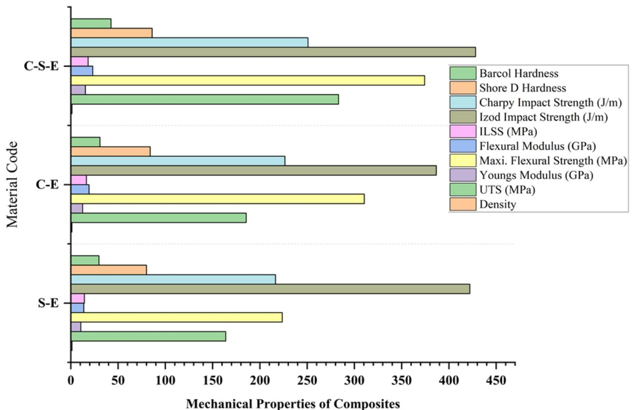
**Fig. 5 Comparison of Mechanical Properties of Composites**
