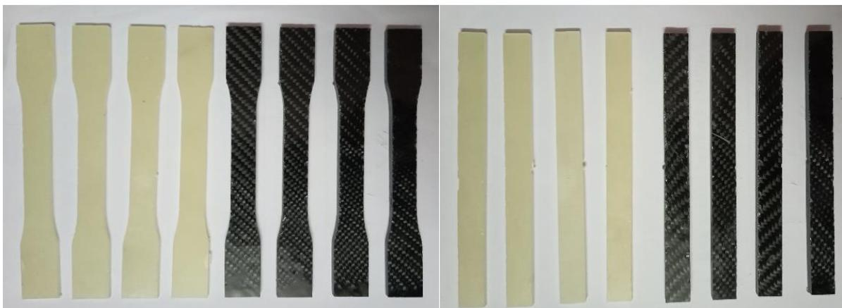
**Fig 4. Abrasive Water Jet Machining & Cut Specimens**
