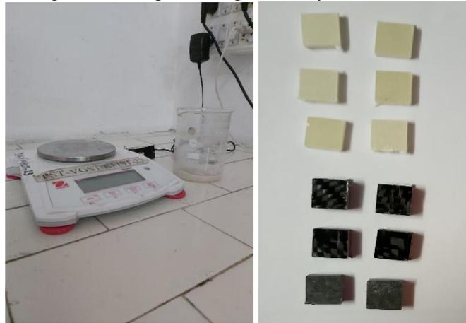
Fig. 6 Density Tester & Specimens
