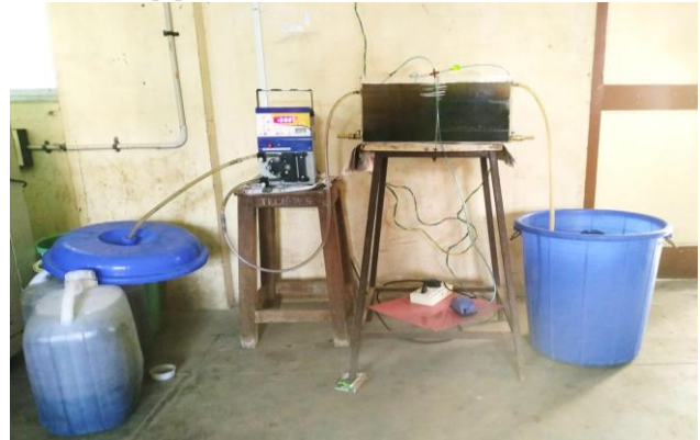
Fig. 1. Photographic outlook of the Aerobic Bio-Reactor
