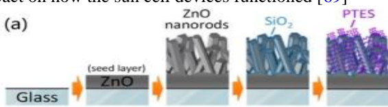
Fig. 14. Perfluorodecyltriethoxysilane (PTES) superhydrophobic SiO 2 -coated ZnO nanorod arrays on glass are prepared as shown in the above figure.
