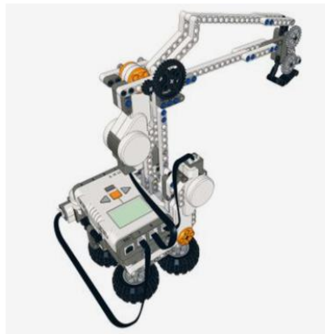
Figure 3.2 Robot arm design(robocamp.eu)
