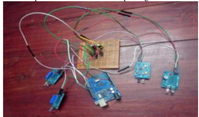
Figure 2: Arduino is connected to 4 IR sensors. The male berg strip is soldered to the PCB which helps to maintain stable power to the capacitors. All the connections made are color-coded
