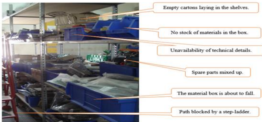
Fig. 1 The warehouse before implementing the 5s methodology
