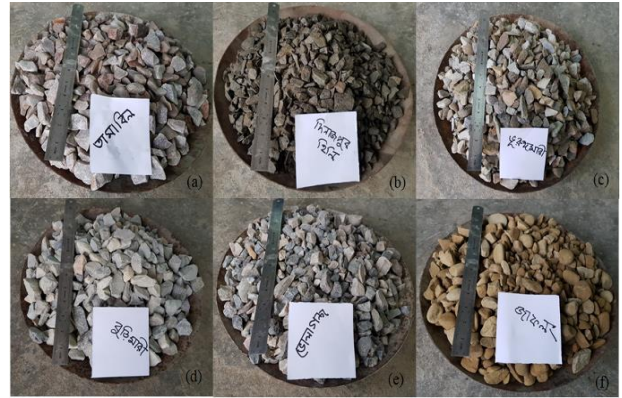
Figure 1: Different types of natural coarse aggregates available in the local market: (a) Tamabil, (b) Dinajpur Hili (Black Stone), (c) Bhurungamari, (d) Burimari, (e) Bholaganj, (f) Jaflong.
