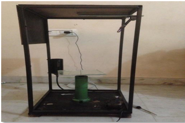
Figure 6: Experimental set up of MR Damper
