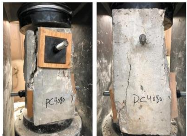
Fig.4: Test setup at the compression testing machine and prism failure.
