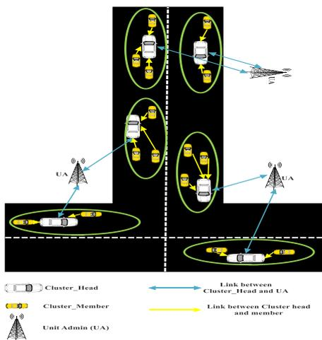
Figure 2: Typical MOVC Model in VANET
