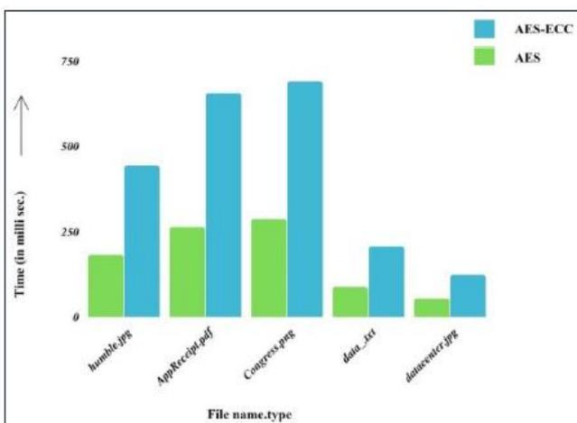
Fig. 16: Graph of Time required for AES and AES-ECC for different file types
