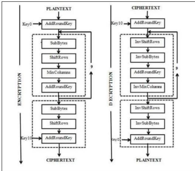
Fig. 7: AES encryption & decryption process[16]
