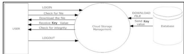
Fig. 10: Data Flow Graph of Recipient User and Cloud Storage Management
