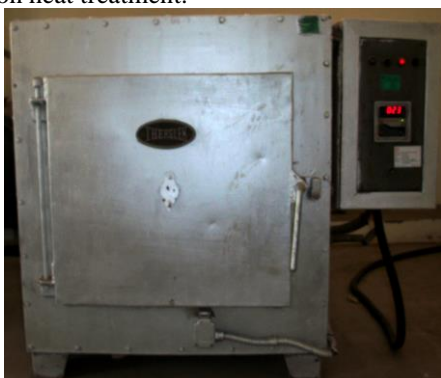
Fig.3 The electric arc heat treatment furnace
