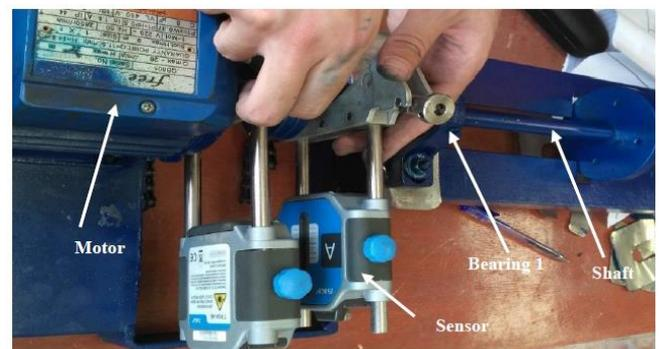
**Fig. 11 Measuring misalignment in horizontal direction.**
