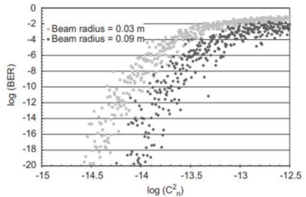
**Fig.1. Typical values of BER versus different turbulent conditions characterized by Cn2 for two initial laser beam radius 0.03 and 0.09 m and laser wavelength 1 ¼ 850 nm for a receiver at distance z ¼ 1000 m. [12]**
