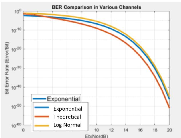
Fig.2. Simulation Of BER vs SNR for Log Normal and Negative Exponential Channel
