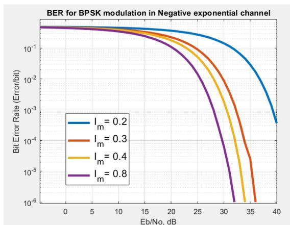
Fig. 4. BER for BPSK modulation in the Negative Exponential Channel.
