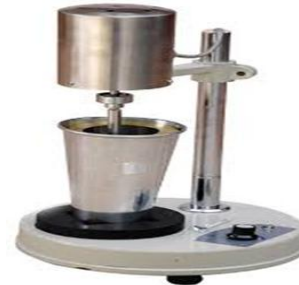
Figure (2): Mechanical Mixer.
